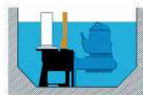
(图一)固定湿式安装 (diagram 1) Fixed wet type mounting
