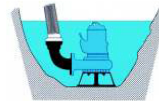
(图三)移动式安装 (diagram 3) Movable mounting
